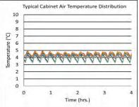
Performance data acquired at 22°C ambient, 4°C nominal set point in an empty cabinet with shelves using air probes, during stabilized steady state operation and a DAQ sampling rate of one measurement every 10 seconds
