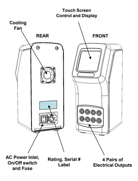
In CONSTANT CURRENT mode, the power supply will output the set mAmp current parameter, and the voltage will fluctuate relative to the resistance of the load (buffer concentration in the attached electrophoresis tanks) up to a maximum of the voltage setting that has been chosen.
