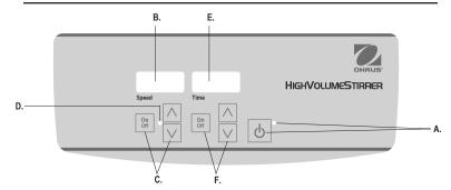
The front panel of the High Volume Stirrer - STHVDG contains all the controls and displays needed to operate the unit.
